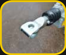
Fig 2 Slide 40mm/50mm towing eye cover over the towing eye.
