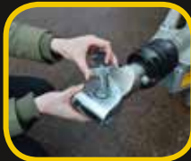
Fig 3 Insert lock bolt body upwards through towing eye lock and towing eye.
