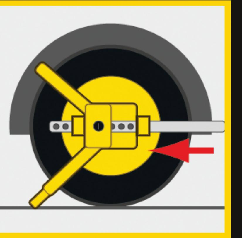
**(2)** Insert the locking arm through the locking plate (in the direction of the arrow), selecting the hole which gives the most secure fit to the wheel (this will depend on tyre width). Push the arm until a tight fit around the wheel is achieved.
