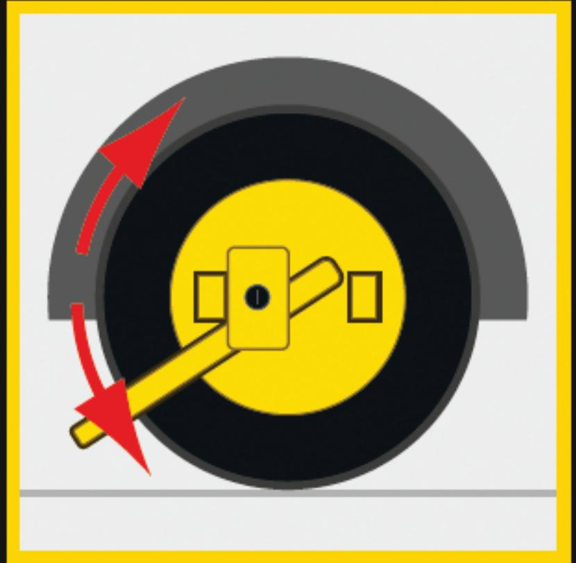
**(1)** Position the arms of the clamp to their maximum open position (in the direction of the arrows shown). Loosely fit the main wheel clamp security plate behind the clamp arms. Position the clamp so the stand rests on the ground. Make sure both tyre arms are tight against the tyre.
