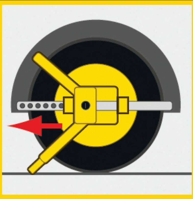
**(3)** With the wheel clamp in position, lock into place using the key. To remove the clamp, unlock with the key, then reverse the process.
